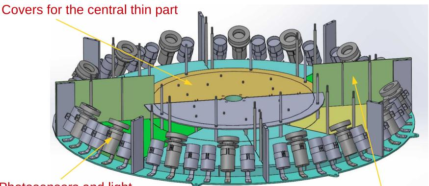
Photosensors and light guide plastic supports. Only for the largest cells we need light guides
