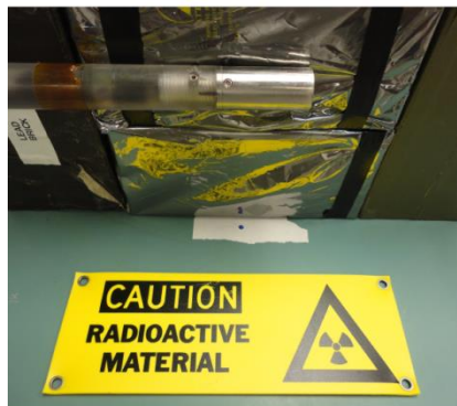
^{252}\text{Cf} neutron source
