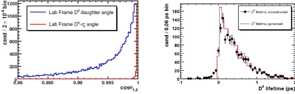
**FIGURE 7.** Left: MC study showing the  $D^0$  daughter angle (blue line) and the  $D^0 - \pi$  angle (redline) in the laboratory frame. As can be seen in the figure, the  $D^0$  and  $\pi$  coming from the  $D^*$  decay are almost collinear. Right: Reconstructed compared to the generated  $D^0$  lifetime using the technique of partial reconstruction of the mother  $B$  meson.
