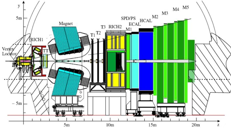
**FIGURE 1.** Schematic representation of the LHCb detector showing its several subsystems. The interaction point is well inside the VeLo, in the left side of the figure.
