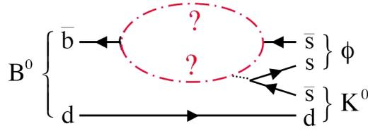
**FIGURE 4.**  $B^0 \rightarrow \phi + K^0$  decay. NP could appear in penguin diagram through the contribution of new particles in loops.
