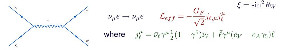
$$\sigma(\nu_{\mu}e \to \nu_{\mu}e) = \frac{G_F^2 s}{\pi} \left[\frac{4}{3}\sin^4\theta_W - \sin^2\theta_W + \frac{1}{4}\right]$$
