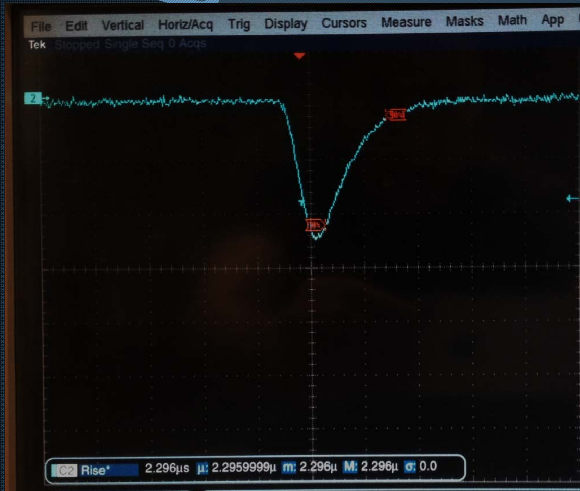
GEM's output signal without RC, with Monitor current.
