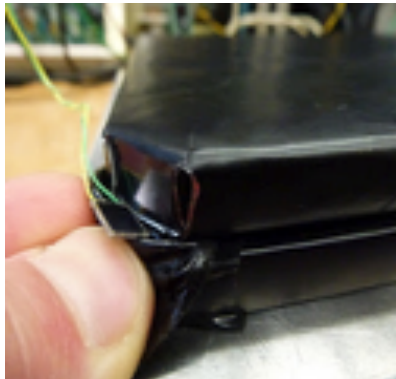
3-Plastic scintillators (EJ-200) and 3-SiPM MicroFC-60035-SMT, SensL
