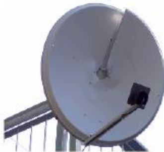
Figure A.4. The helicoidal parabolic antenna.
