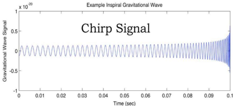
The shrinking will make GWs increase in frequency and amplitude.
