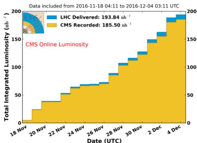
Cumulative luminosity measured online versus day delivered to, and recorded by CMS during stable beams and for p-pb collisions at 5 TeV and 8 TeV centre-of-mass energy in 2016.
