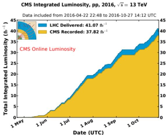
Cumulative luminosity measured online versus day delivered to, and recorded by CMS during stable beams and for p-p collisions at 13 TeV centre-of-mass energy in 2016.
