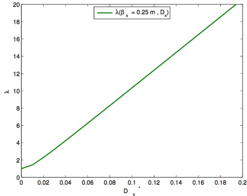
Figure 6.1: Monochromatization factor versus  $D_x^*$  at fixed  $\beta_x^* = 0.25 \text{ m}$ , for constant emittance and energy spread.
