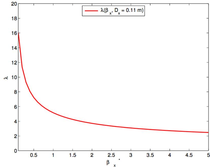
Figure 6.2: Monochromatization factor versus  $\beta_x^*$  at fixed  $D_x^* = 0.11 \text{ m}$ , for constant emittance and energy spread.
