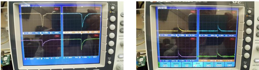
**Figure 12.** Left, signals obtained with positive high voltage. Right, signals with negative high voltage. They are slower compared with those from positive high voltage.
