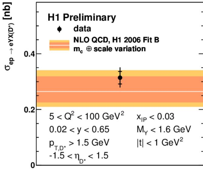
**NLO QCD prediction agree well within errors with measured cross sections**
