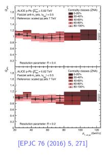
•  $p_{\perp}$  spectra for charged jets: anti-kt,  $|\eta| < 0.5$ , R = 0.4 (top), R = 0.2 (bottom)
