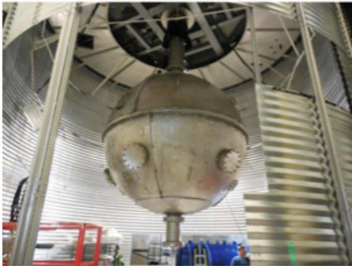
Steel Shell in shield tank
