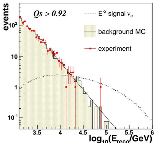
Figure 3: The reconstructed cascade energy distribution  $E_{\text{reco}}$ . Shown are experimental data as well as background and signal Monte Carlo simulation after application of all quality cuts and a cut on the discriminating parameter  $Q > 0.92$ . The smooth line is a result of the power-law fit to the background simulation.
