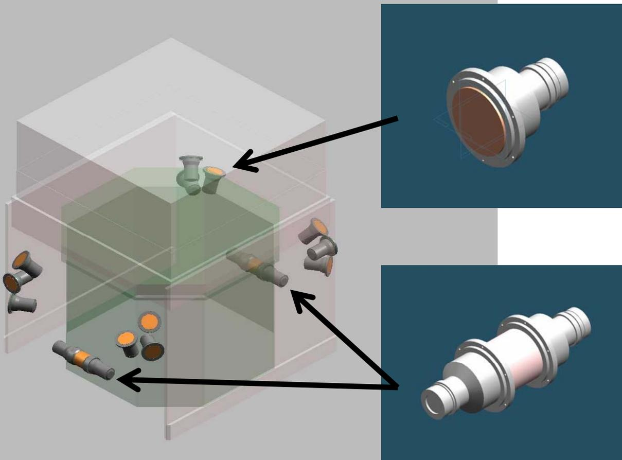
*12 Sodium Iodide (NaI) scintillation detectors*
