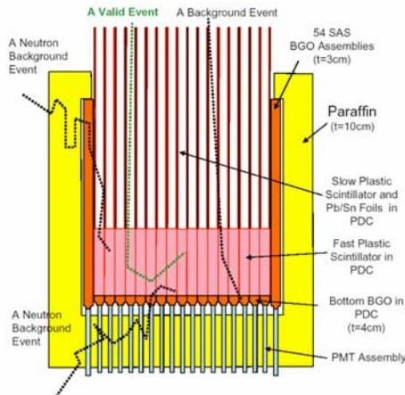
Figure 2: Schematic cross section of the PoGOLite instrument (not to scale) showing valid and background photon interactions. Possible background atmospheric neutron interactions are also shown.
