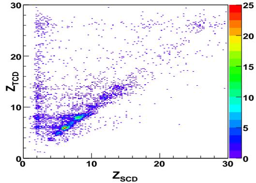
Figure 1: SCD versus TCD charge for events passing through the full TCD-TRD-SCD stack. Identically identified charges lie along the diagonal, with B, C, N, and O most prominent. All remaining events lie in the reasonable region of lower SCD than TCD charge. Events along the TCD-identified C and O lines correspond to charge-changing interactions within the instrument.
