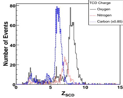
Figure 3: TCD-identified O, N, and C with good tracks in the TCD and SCD active areas correspond to their SCD-determined charge. TCD O fragmenting to N and C events are also visible. The latter are more prevalent due to resonance at alpha emission.
