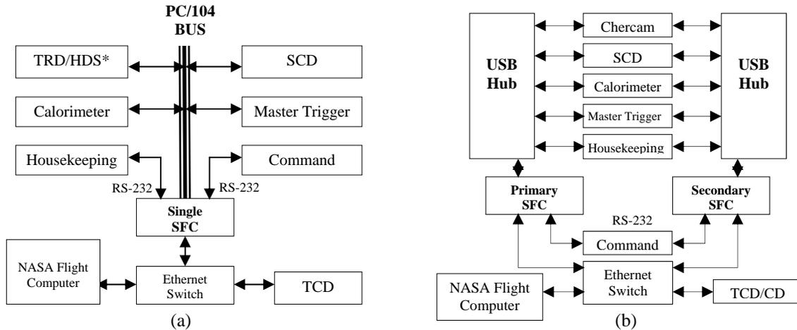
Figure 1: Comparison of CDAQ system architectures (a) CREAM-I/II (\*only for CREAM-I) (b) CREAM-III.
