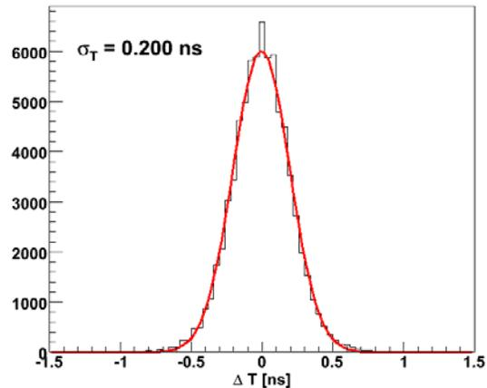
Figure 3: Timing resolution of a single S11 paddle for protons
