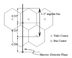
Figure 1: Example of relative size of angular bins on the photomultiplier tube cluster face.
