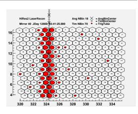
Figure 2: Typical vertical calibration laser shot as seen by HiRes2 from the night of 30 January 2003. Note that there are many more time bins than angular bins. Here angular bin centers are separated by  $1.5^{\circ}$ .
