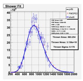
Figure 3: Example of a monte carlo generated air shower and the fit to the shower profile. The abscissa is depth in  $g/cm^2$  and the ordinate is the number of charged particles. Diamonds are the thrown shower profile, squares are the reconstructed shower profile and the solid line is the Gaussian in age fit found to best match the shower.
