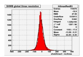
Figure 6: Xmax resolution of monte carlo simulated showers representative of the entire lifetime of stereo operations at HiRes. The resolution is seen to be  $32.3 \text{ g/cm}^2$  for events with reconstructed energy greater than  $10^{18.5}$  eV.
