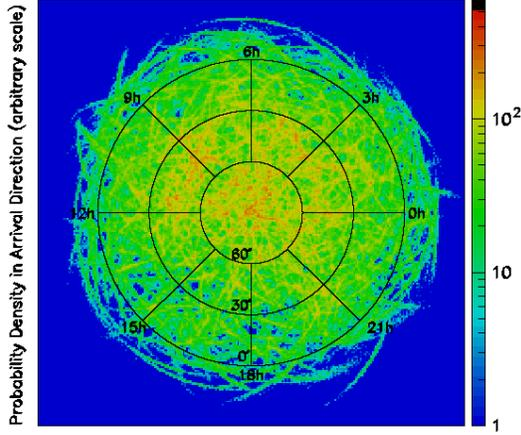
Figure 1: Skymap of arrival directions of events in the the HiRes-I monocular data set, plotted in polar projection, equatorial coordinates. Angular bin size varies across the map, but averages  $1^\circ \times 1^\circ$ . Each event is represented by 1,000 points randomly thrown according to the elliptical Gaussian error model of Equations 1 and 2.
