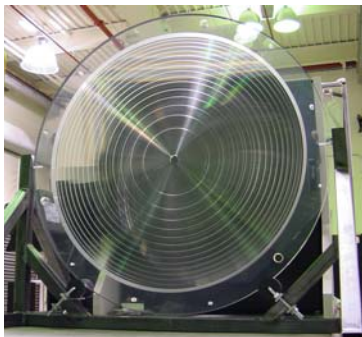
Figure 2: A prototype model of the Fresnel lens of the JEM-EUSO telescope with a diameter of 1m.
