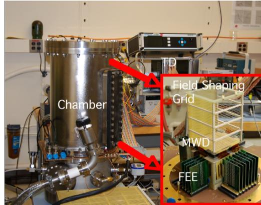
Figure 2: Prototype 3-DTI detector for characterization of  $10 \times 10 \text{ cm}^2$  MWD performance. Shown here is a MWD, drift electrode,  $15 \text{ cm}$  field-shaping grid, and 16-channel FEE cards.
