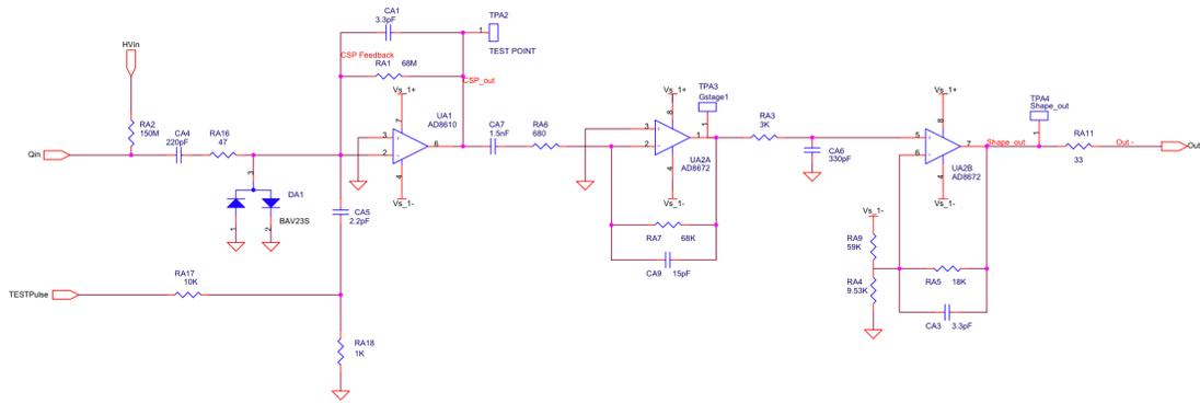
Figure 1: The schematic of a front end electronics channel. It shows a charge sensitive preamplifier and CR-RC pulse shaper.
