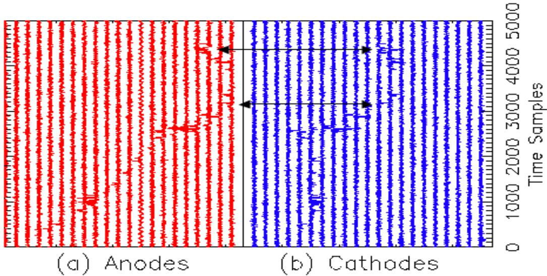
Figure 3: The raw TD output of the ionization charge recorded from a pair production event for (a) the anode strips and (b) the cathode strips versus sampling time. Only a portion of the active MWD anodes and cathodes are shown here for clarity.
