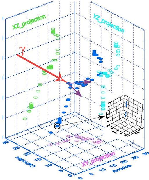
Figure 4: Reconstruction of the raw data (Fig 3). The arrows indicate our best estimate of the electron-positron directions (purple) and incident gamma ray direction (red). The inset figure shows the individual ionization charges at the full time resolution of the TD.
