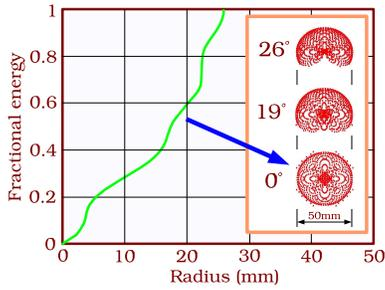
Figure 2: Optical spot (produced by paraxial beams) on mosaic surface with mosaic shadow
