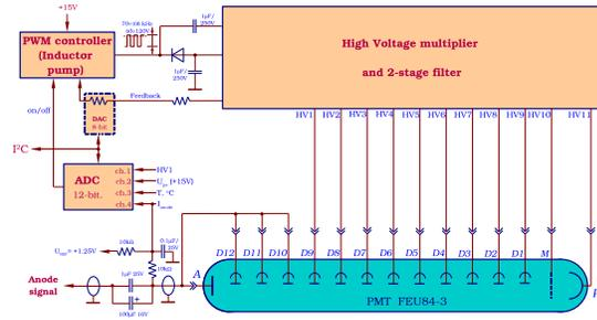
Figure 3: High voltage power supply for optical module
