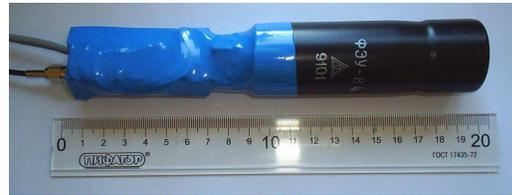
Figure 4: Optical module. PMT with High voltage power supply
