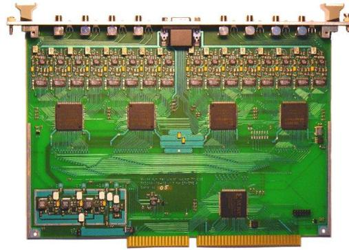
Figure 6: 8-channel FADC board
