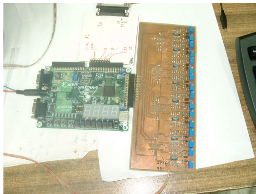
Figure 8: Daughterboard used to provide a reference signal for each analog output of the PMTs and to convey the LVDS-like pair of signals into the LVDS inputs of the FPGA.
