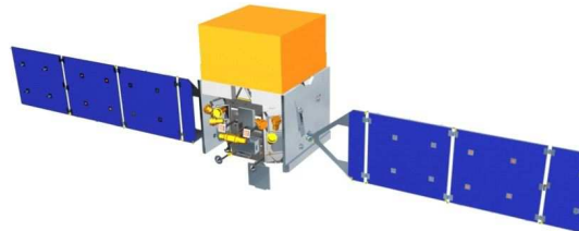
Fig. 7. Schematic of the GLAST satellite deployed in orbit. The LAT , which comprises of a cluster of 16 silicon strip trackers and a calorimeter consisting of 8 layers of CsI(Tl) crystals, is in the top (yellow) area; the Gamma Ray Burst Monitors GBM are located directly below.
