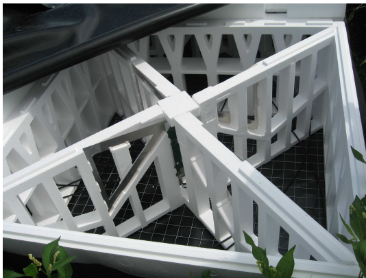
Fig. 5. Inside of a LOFAR High-Band Antenna (HBA) tile, showing one crossed bow-tie antenna.
