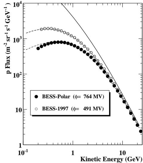
Figure 1: BESS-Polar I proton flux compared with the proton flux of BESS(97) (lines see text).
