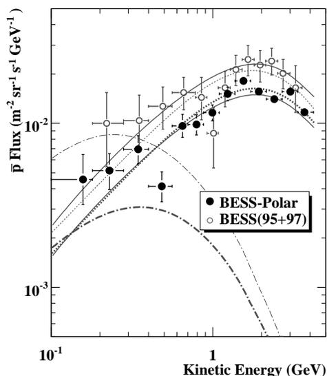
Figure 2: Antiproton spectrum measured in BESS-Polar I compared with BESS(95+97) results (lines see text).
