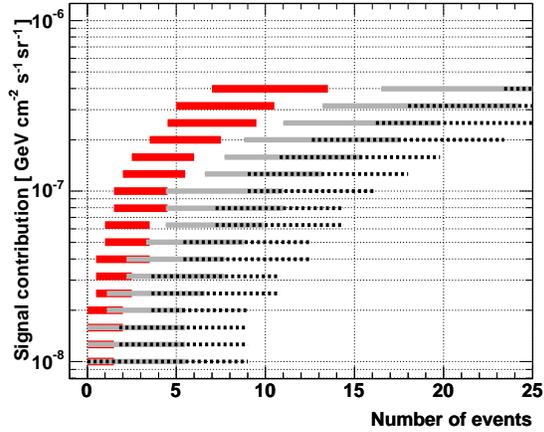
Figure 4: The unified approach of Feldman and Cousins has been applied to the unfolding problem by calculating individual probability density functions. 90% Feldman-Cousins confidence belts of three unfolding energy bins: 50 to 100 TeV (black dotted), 100 to 300 TeV (gray) and 300 TeV to 1 PeV (red) are displayed.
