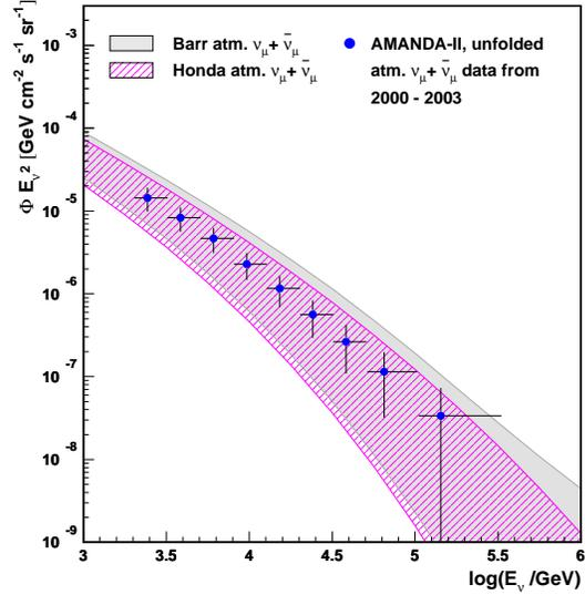
Figure 2: Comparison of the unfolded energy spectrum with flux expectations according to Ref.[6, 7]. The shaded bands show the range between the horizontal (upper border) and vertical flux (lower border).
