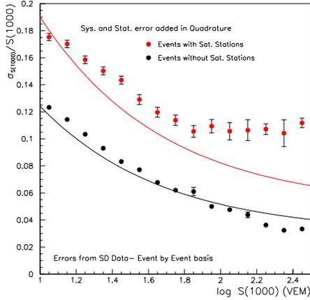
Figure 5: Total error in  $S(1000)$  calculated on an event by event basis from the data. The data is separated in two sets: events with (without) saturated stations. The lines correspond to the predictions from full MC calculations (see text for details)
