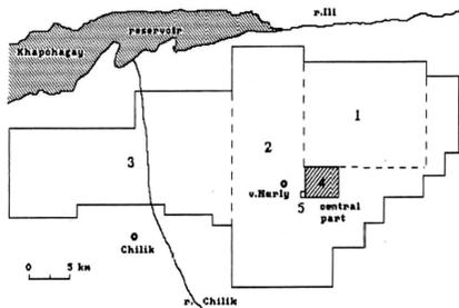
Fig. 2. The EAS-1000 installation. 1 -  $S = 100 \text{ km}^2$  — first stage array,  $L = 500 \text{ m}$ , 2 -  $S = 500 \text{ km}^2$  — half of the array with  $L = 500 \text{ m}$ , 3 -  $S = 500 \text{ km}^2$  — expanded array,  $L = 500 \text{ m}$ , 4 -  $S = 20 \text{ km}^2$  — central part,  $L = 70 \text{ m}$ , 5 -  $S = 2 \text{ km}^2$  — prototype,  $L = 500 \text{ m}$ .
