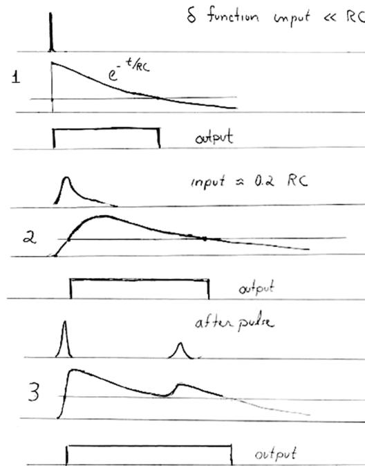
Fig. 14. Three possible situations for a logarithmic charge to time converter.
