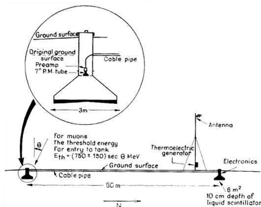
Fig. 16. Arrangement of an individual detector in the Sidney array.
