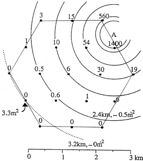
Fig. 8. The Volcano Ranch Array. The densities for the 10<sup>20</sup> eV event are shown.
