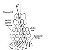
FIG. 1. Projection of the aperture of the optical detector onto a vertical plane above the center of the Volcano Ranch scintillator array. A reconstructed shower trajectory is indicated by the heavy line. Crosses denote phototube apertures in which a signal was detected.
