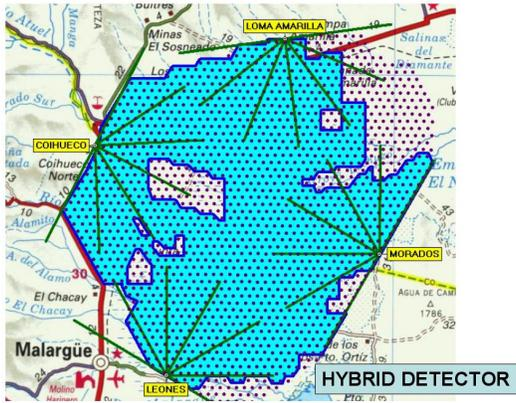
Fig. 32. Plan of the Auger Observatory. Completed surface array is outlined in blue. The location of the fluorescence detectors is indicated in yellow.
